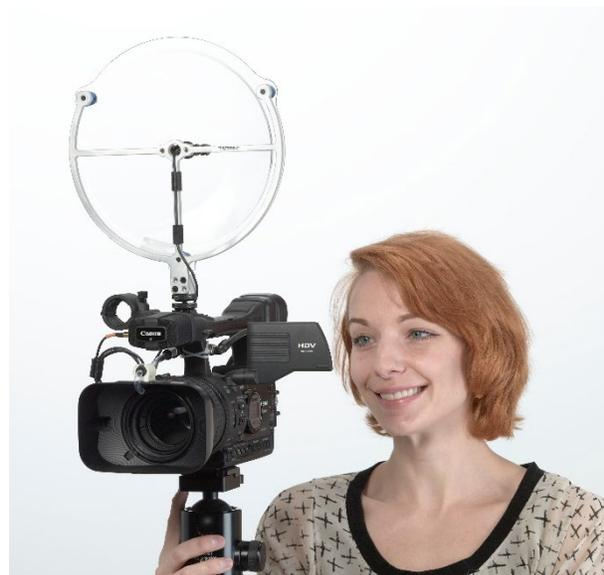
Any omni-directional lapel microphone can be used in the 9-inch parabolic, so it works with any camera with a microphone input. The base of the parabolic mic's frame incorporates a 1/4-20 thread so it can be used in a multitude of ways. It can be mounted to the cold shoe of a camera, or to a small pistol grip handle and hand-held. If required, the small parabolic microphone can be mounted to a light stand, placed on the end of a boom pole or suspended from the ceiling grid in a studio.
